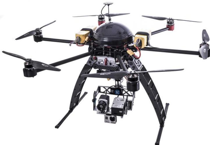
Remote Aerial Surveys collected the data using a small UAV, a XM6 Qi-TR (our current operational platforms can be legally flown in wind speeds up to 17mph, and at heights up to 400ft.) The UAV had a Panasonic Lumix GH3 camera attached. On site it was the responsibility of the pilot to assess local weather conditions to decide whether the flight was safe. As required by regulation the platform was operated within line of sight of the pilot, or within 500m, whichever is was lesser of the two.
